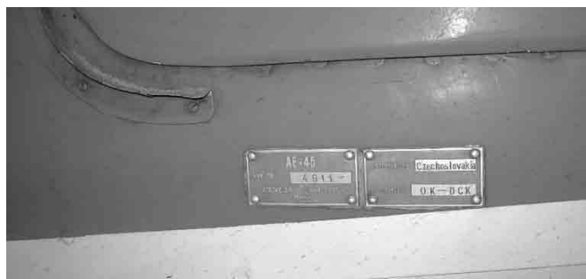
The construction plate is at the left side of the lower fuselage just in front of the wing root.
