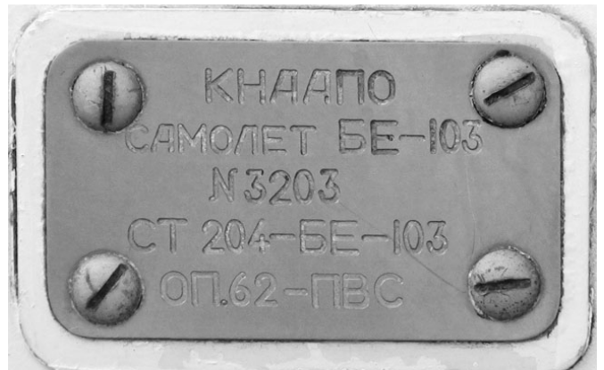
The construction number plate is on the left rear side of the fuselage below the rear end of the left engine.
