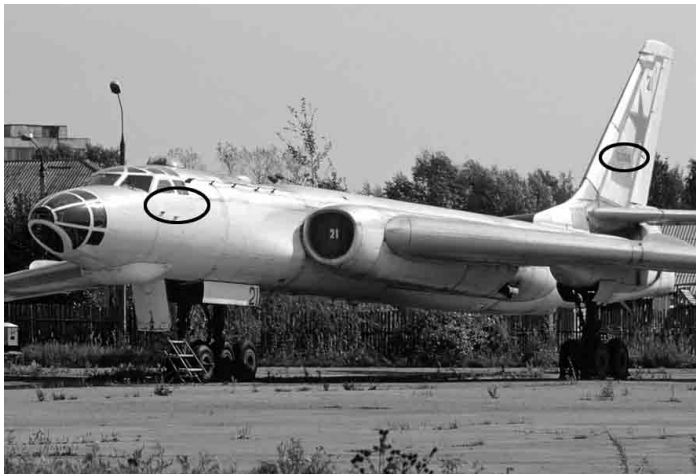
The Tu-16 construction number is normally painted on the nose and tail on both sides.
