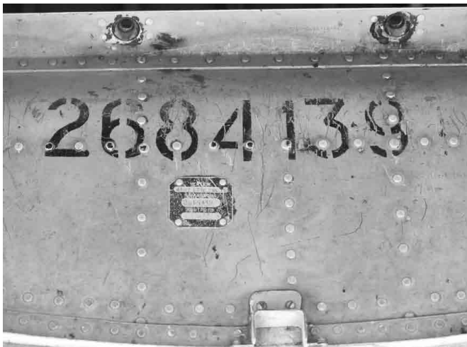
The construction number is painted in the bomb bay, visible when looking to the rear. It can also be found on the rear wall of the nose-wheel bay. Sometimes painted on and sometimes on a tiny plate (with the drawing number starting with 145 in the upper line and the construction number on the lower line). Apart from that, the construction number can be found on the plate of the nose-wheel strut (in the right upper corner of the plate).
